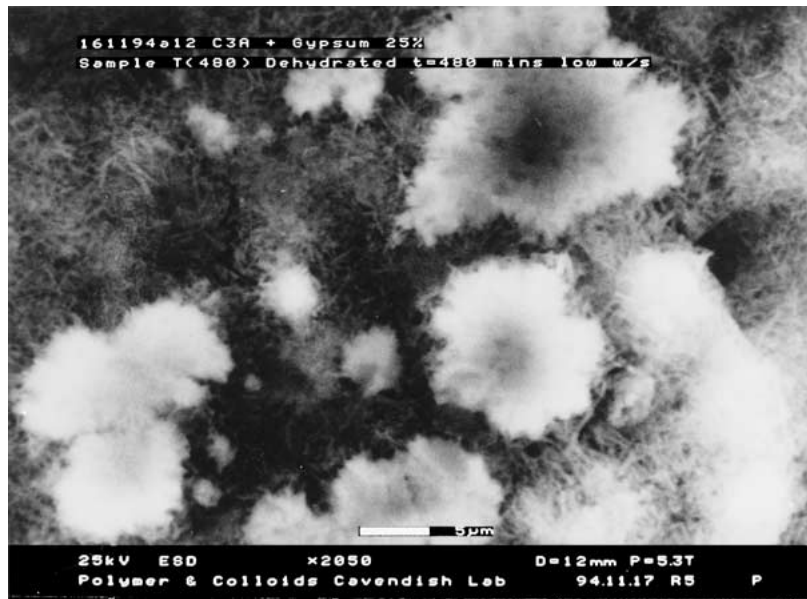
Figure 7 Irregular platelets of secondary monosulphate forming from bundles of ettringite needles after eight hours hydration. W/S = 5, %gypsum = 25. Scale bar is 5 μm.
