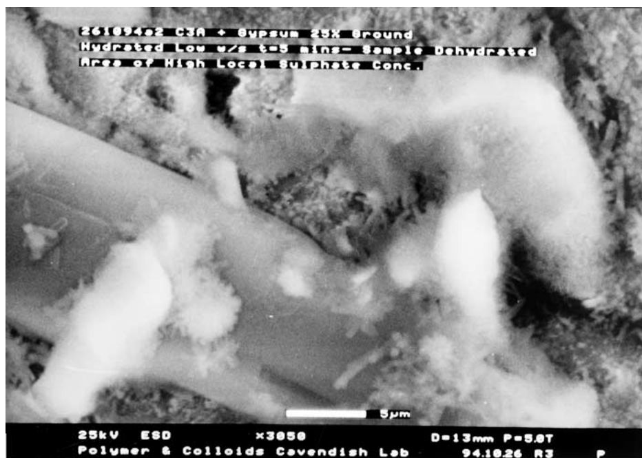
Figure 5 Short stubby ettringite crystals developing proximal to large gypsum crystals. Image taken after five minutes hydration. W/S = 5, %gypsum = 25. Scale bar is 5 μm.
