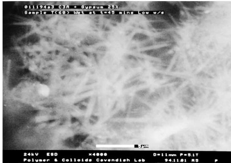
Figure 9 Long slender ettringite crystals growing in an intergranular space. W/S = 10, %gypsum = 25. Scale bar is 5 \mu\text{m} .
